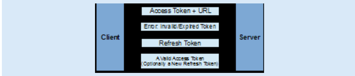
Figure 3.4: Accessing a protected resource with an invalid access token in OAuth 2.0
